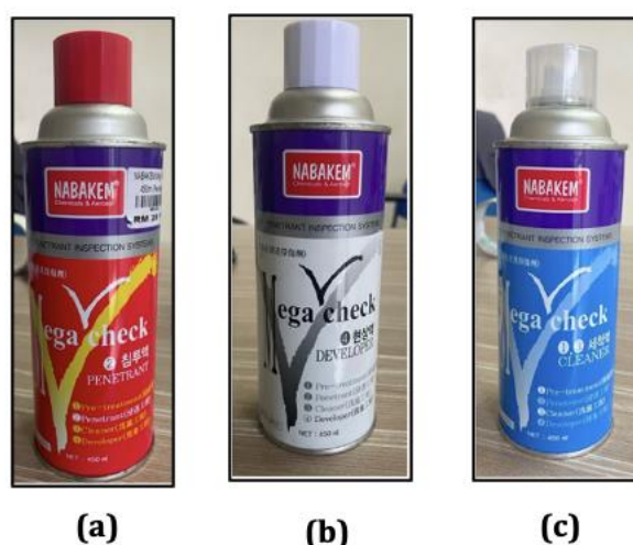
Fig 5 (a) Red Dye Penetrant; (b) Developer; (c) Cleaner Solvent
