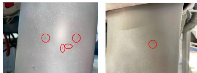
Figure 12 Flaws on Propeller Blade
