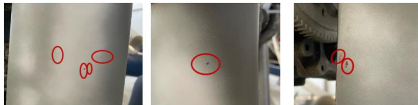
Fig 14 Flaws detected on Propeller Blade
