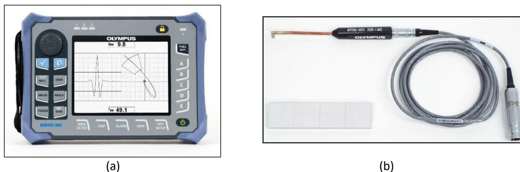
Fig. 5 Eddy current testing equipment used in this study: (a) Olympus Nortec 600 flaw detector and (b) right-angle flexible metal shaft surface probe.
