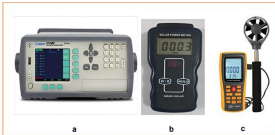
Fig. 3. a) digital data logger (AT4532), b) solar power meter SM206, c) GM-8902 anemometer
